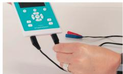
Due to the fit of the electrode sets included as accessories, the connection is protected against reverse voltage. Only use original accessories.
