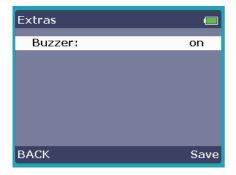
This menu item allows you to switch the beeps on and off. To do this, use parameters buttons + and - and confirm the setting with button 3 • "Save".
