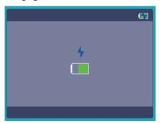
The voltage of the battery is shown on the display in the header on the right by means of an icon.
